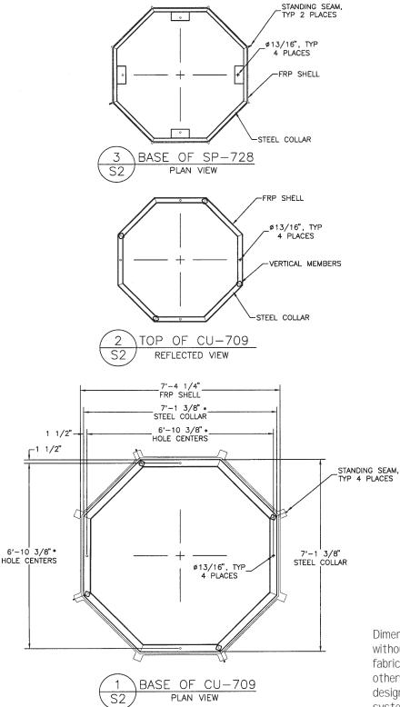
Dimensions and details are subject to change without notice. All cupola and steeple units are fabricated using minimal standing seams unless otherwise noted. All cupola and steeple units are designed to be erected on a completed roofing system and are not guaranteed to be leak proof.
